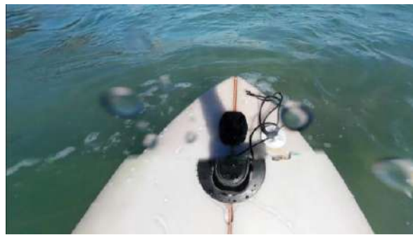
Figure 2. 360-degree camera image hiding the camera but showing stitch imperfections
