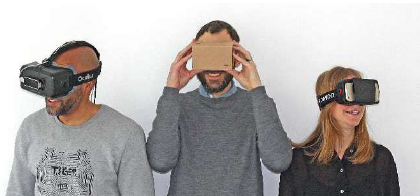
Figure 4. Examples of three different head-mounted displays. Oculus Rift developer kit 2 to the left, Google Cardboard used with a smartphone in the middle and Homido used with a smartphone to the right.
