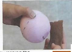
A polystyrene sphere is made by rasping the overall shape, followed by successively finer grades of sandpaper and a sanding template.
