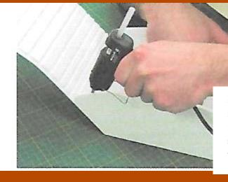
Front Panel Step 3 Attach the side pieces to the rear piece with hot glue. Apply the glue to the rabbet cut and hold while glue dries. Attaching the sides to the back first will make it easier to attach the curved front piece.
