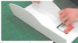
Front Panel Step 2 Rabbet cuts are made on each side of the front piece to accept the two side pieces and hide the edge of the foam. The front piece is then scored with V-notches on the inside at 1cm (0.4in) intervals to allow the surface to curve.
