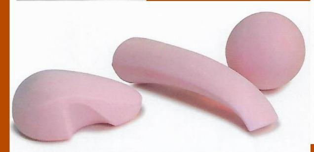
There are two different kinds of polystyrene foam. Extruded foam (XPS) – or Styrofoam – is a readily available solid insulation material sold in various thickness sheets by builder's merchants. Depending on the supplier, it will be manufactured in different colours, including pink, blue or white. It may also be purchased as thicker pallets from specialty suppliers. The low density of the material 40kg/m3 (2lb/ft3) makes it extremely easy to work with.
