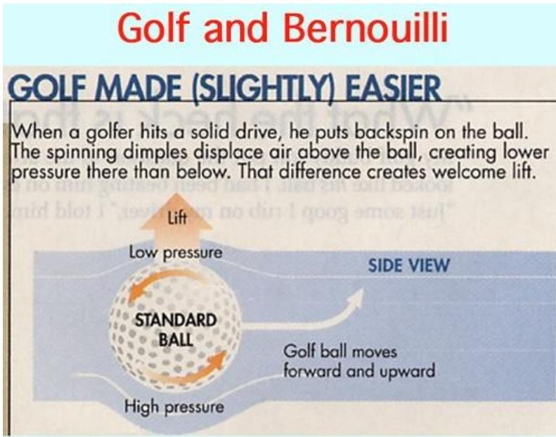
$$Z_0 + \frac{P_0}{\gamma} + \frac{V_0^2}{2g} = Z_S + \frac{P_S}{\gamma} + \frac{V_S^2}{2g}$$
