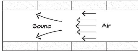
Under FORWARD FLOW conditions, high-frequency sound is refracted toward the duct walls.
