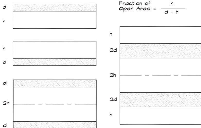
**FIGURE 14.3 Attenuation in a Lined Duct (Beranek and Ver, 1992)**
