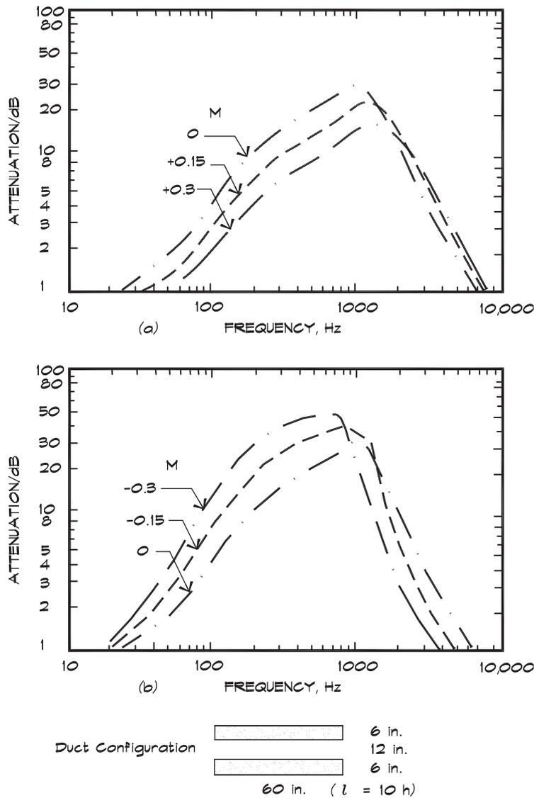
of the duct. The gradient refracts the high frequency energy toward the duct walls yielding somewhat greater losses for propagation in the downstream direction. Figure 14.4 shows this effect.
