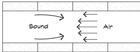
Under REVERSE FLOW conditions, high-frequency sound is refracted away from the walls and toward the center of the duct.
