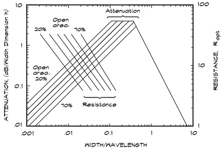
Relationship between the optimized liner resistance and the maximum attenuation that can be achieved for the fundamental mode in a rectangular duct with one side lined with a locally reacting porous liner. The left axis is the attenuation in a length of duct equal to the air channel width  $h$  and the right axis is the optimum value of the normalized flow resistance.
