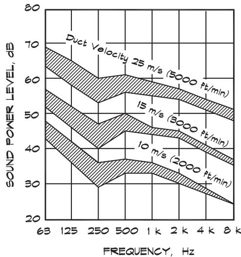
**FIGURE 13.17 Buffeting in Rectangular Ducts (Fry, 1988)**
