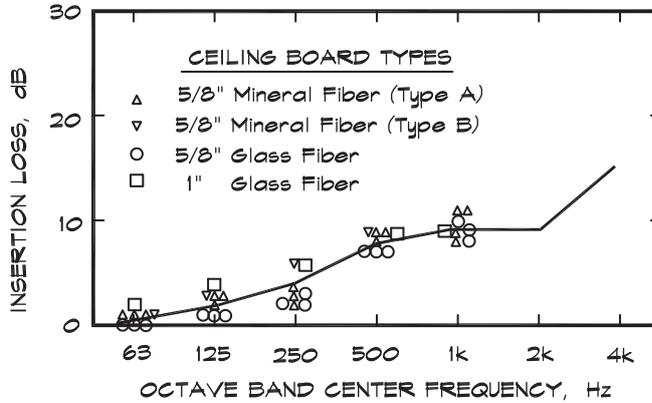
discrepancy may be due to the difficulty in duplicating in the field the smooth entry and exit flow conditions under which the laboratory data are taken. Blazier (1981) has also measured the insertion loss due to acoustical tile ceilings given in Fig 13.15. Note that the loss approaches 10 dB only at high frequencies.
