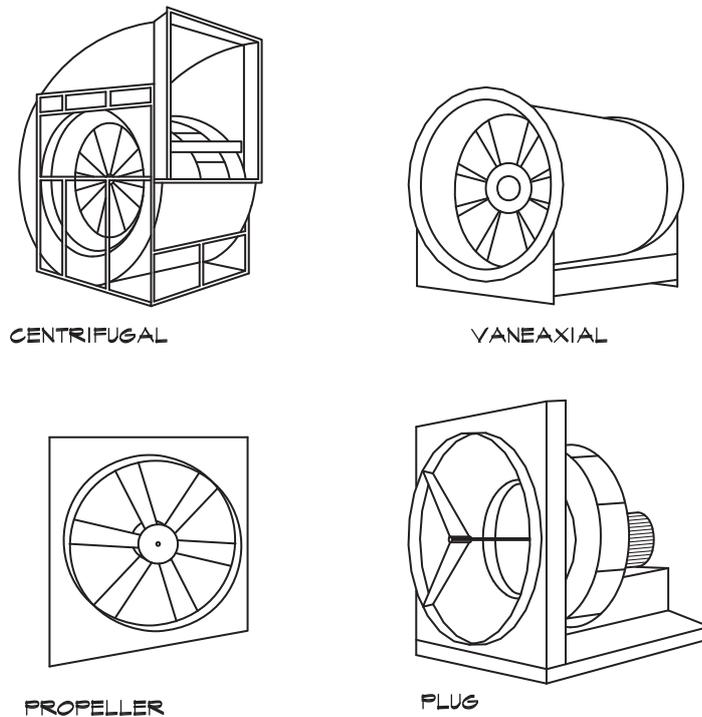
FIGURE 13.8 Types of Centrifugal Fans
