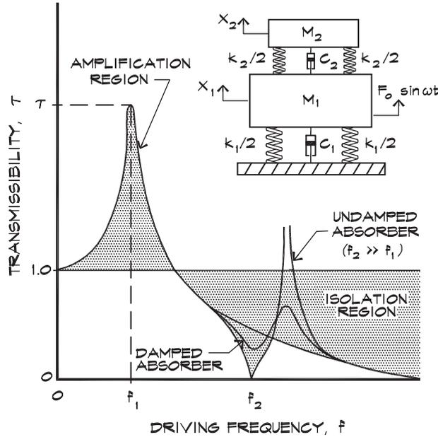
**FIGURE 11.20 Forced Response of a Two Degree of Freedom System Near Resonance (Ruzicka, 1971)**
