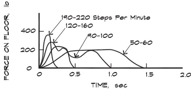
**FIGURE 11.30** Dependence of the Maximum Force  $F$  and the Rise Time  $t$  of a Footstep Pulse on the Walking Speed (Ungar and White, 1979)
