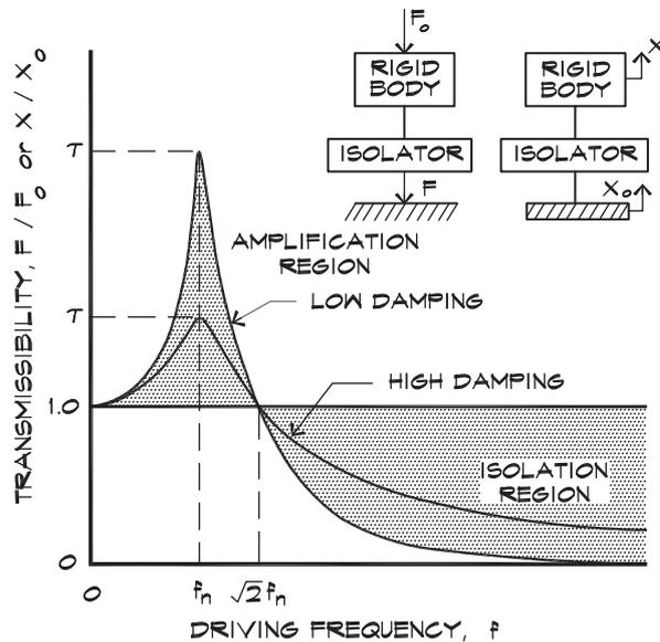
from below. The transmissibility is the same as that given in Eq. 11.23. In the case of isolated equipment, instead of the force being generated by a vibrating machine, a displacement is created by the motion of the supporting foundation. In Eq. 11.23 the terms for force amplitudes are replaced by displacement amplitudes.
