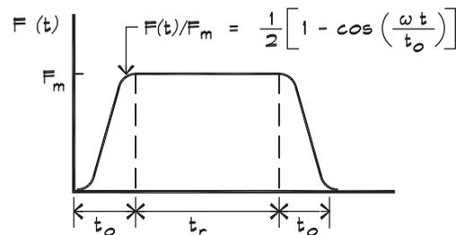
FIGURE 11.28 Maximum Dynamic Deflection Due to a Footstep Pulse (Ungar and White, 1979)
