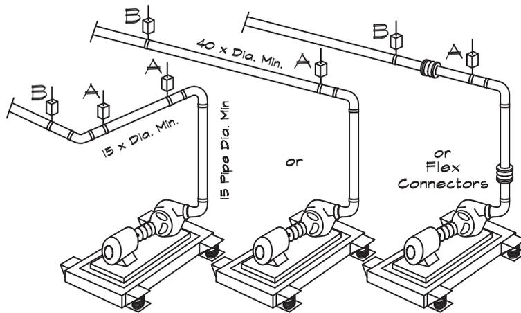
Each of the above alternatives will result in equivalent piping isolation from a flexibly supported pump if the following suggestions are implemented.
