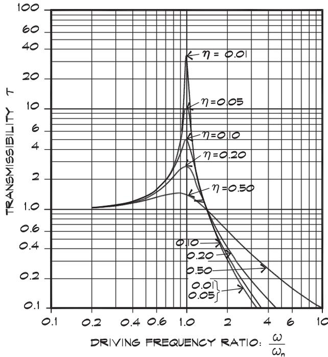
Figure 11.7 shows a plot of this expression in terms of the transmissibility, which is the ratio of the transmitted to the imposed force. We can see that above a given frequency ( $\sqrt{2} f_n$ ), as the frequency of the driving force increases, the transmissibility decreases and we achieve a decrease in the transmitted force. This is the fundamental principle behind vibration isolation.
