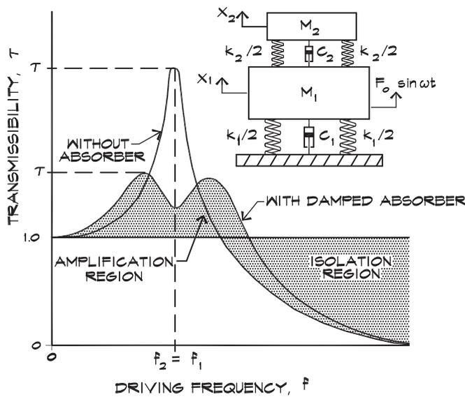
relevant floor area, are hung between the ceiling and the slab. It is not advisable to use the ceiling itself as the dynamic absorber, since mass damping works to minimize floor motion by maximizing the motion of the suspended mass. If the ceiling motion is maximized, it will radiate a high level of noise at the floor resonance.
