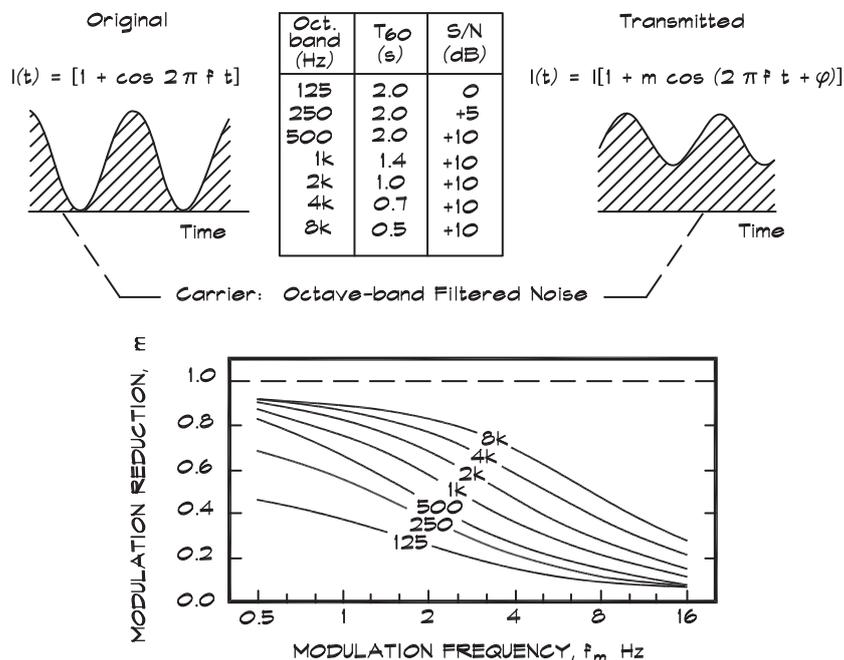
Illustration of how an MTF analysis is performed by using an octave-band filtered noise carrier, 100% intensity modulated, for each modulation frequency successively. This leads to a family of MTF curves. Each curve is calculated for the data given in the table.
