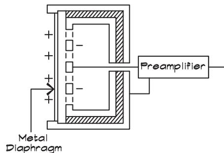
become a capacitor when a DC polarizing voltage, typically 150 to 200 V, is applied. Motion of the diaphragm generates an electrical signal by varying the capacitance and thus the voltage between the plates. These microphones are very sensitive and accurate and have excellent frequency response characteristics. They are less rugged than dynamics and require a source of the polarizing voltage.
