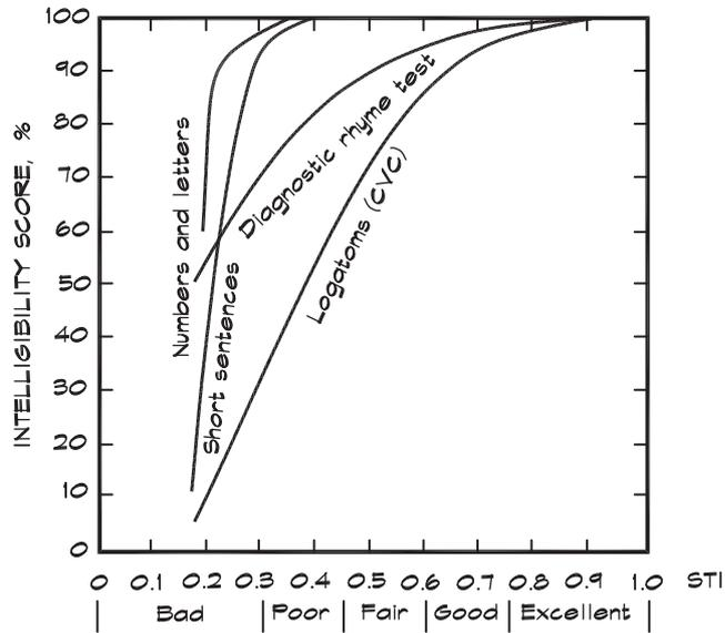
FIGURE 4.30 A Comparison of Articulation Index and Speech Transmission Index (Houtgast et al., 1980)
