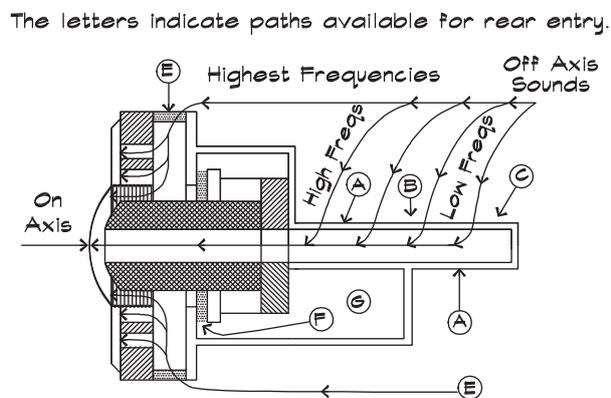
Highly directional microphones can be made using a series of openings in a tube, or a group of different length tubes, leading to the diaphragm. These so-called shotgun microphones work because sounds arriving on axis and entering through the holes combine in the tube in the proper phase relationship. Sounds arriving from the side and traveling down the tube combine with a random phase relationship that attenuates the signal at the diaphragm.
