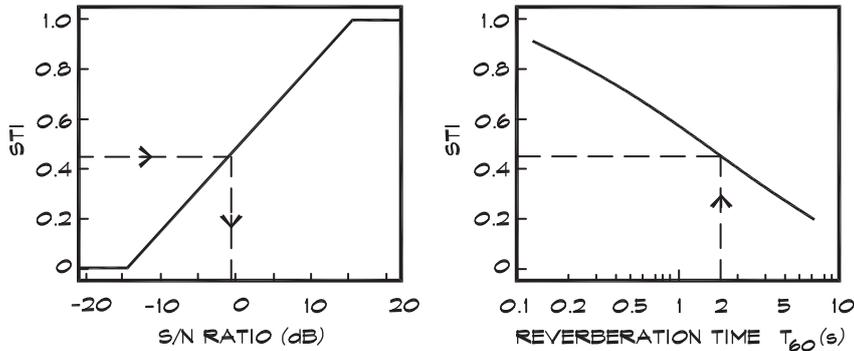
The dashed curves below represent the traditional approach in which the equivalent S/N ratio is defined by the ratio between the early and the late part of the energy time curve.
