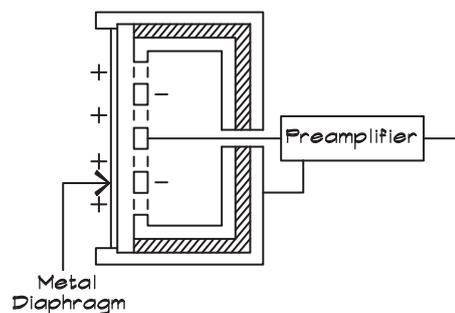
become a capacitor when a DC polarizing voltage, typically 150 to 200 V, is applied. Motion of the diaphragm generates an electrical signal by varying the capacitance and thus the voltage between the plates. These microphones are very sensitive and accurate and have excellent frequency response characteristics. They are less rugged than dynamics and require a source of the polarizing voltage.
