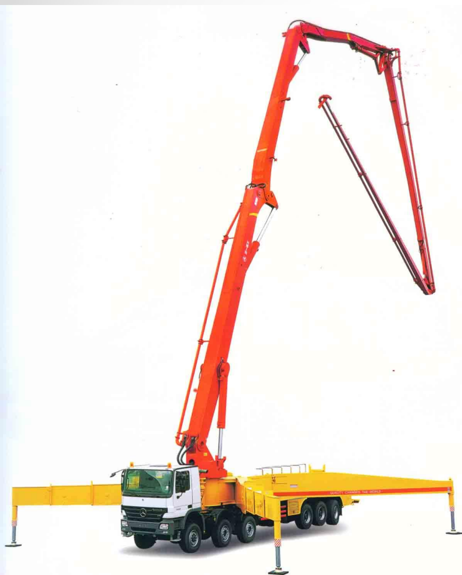
mobile concrete pump
