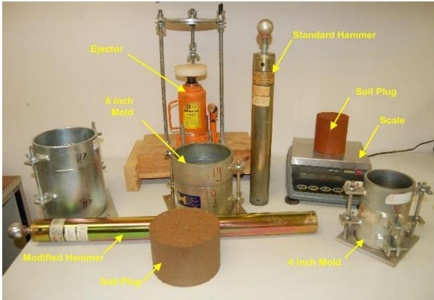
Typical Proctor Test Equipment
