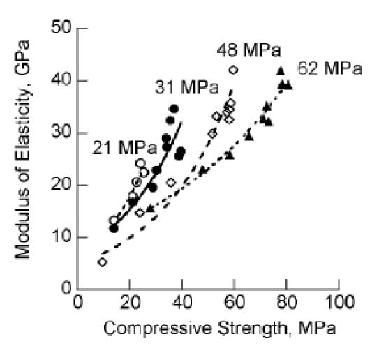
Quality and Quantity of agregat → significant effect on elasticity
