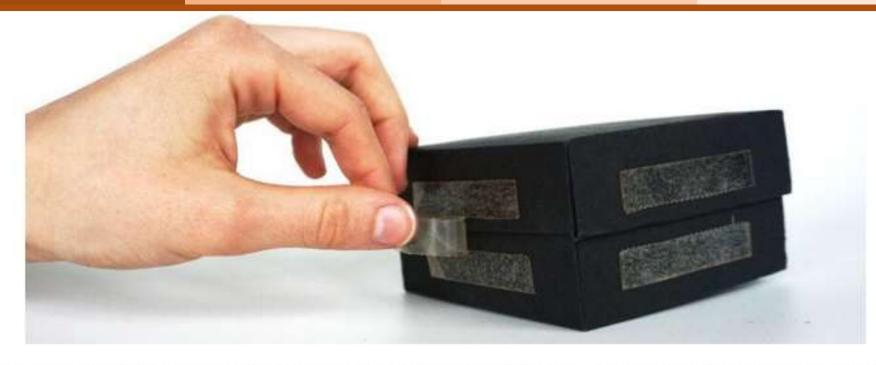
The result is MarinaTex, a bioplastic film made primarily from fish scales and skins and bound with an organic binder. Creating MarinaTex required a lot of trial and error, but the result is more than a polymer; MarinaTex is biodegradable plastic sheeting that is versatile and naturally decomposes in 4 to 6 weeks in a home **compost** environment.
