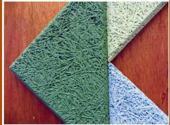
The acoustic and thermal panels from Sweden's Baux are made of wood, wool and cement, natural components that are both environmentally friendly and recyclable.
