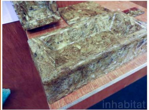
Spyros Kizis created cast bricks made from artichoke thistles and bio-resin from waste cooking oil. The artichoke head is combined with epoxy resin and then cast in a mold to achieve the desired shape.
