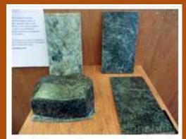
collects Solidwool from wool sheep farmed in the upland areas of the UK to create a beautiful and tough composite material. Low carbon footprint bio resins are used in the production make process to Solidwool sustainable alternative to fibreglass.
