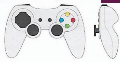
Step 1 The process starts with sketching the form of the product. Scale top and side views will be used as cutting templates. These can be hand-drawn or created in Illustrator®.
