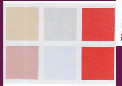
Low-density PU foam shows porosity when primed and painted (top row), whereas high-density PU foam is smooth when painted (bottom row).
