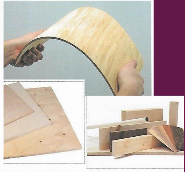
Plywood (above) is made in different grades for different applications. Bendy or flexi-plywood (left) is a useful material for creating curved planes in wood.
