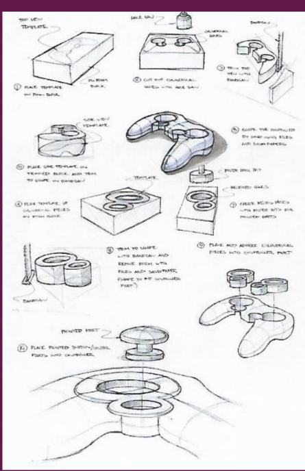
Step 3 The top outline of the game controller is glued on to a piece of PU foam that has been trimmed to the overall thickness. The cylindrical control housing outlines will also be cut from the same piece of foam.
