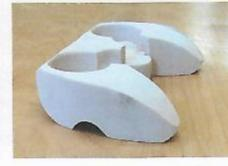
**Step 9** The finger-rest concave surface is sanded with a post sander. This could also be done with a circular-shaped rasp.
