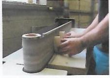
Step 8 The side profile is then sanded to shape on a belt sander. This could have been done with a hand-held rasp instead, in which case the part would be mounted in a vice while being worked on.
