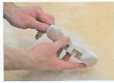
**Step 10** The shape is now sanded manually, blending the surfaces into a final desired shape.
