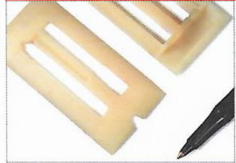
Fine-detail CNC-machined ABS prototype. These parts were machined with a very fine-ball end-mill cutter (1.5mm/0.06in dia.).
