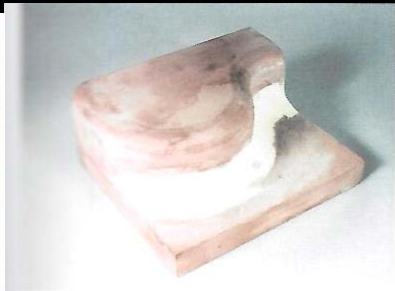
Step E The final shade should feel smooth and is then ready for priming. Half of the block has been painted to show what the form will look like. A few coats
