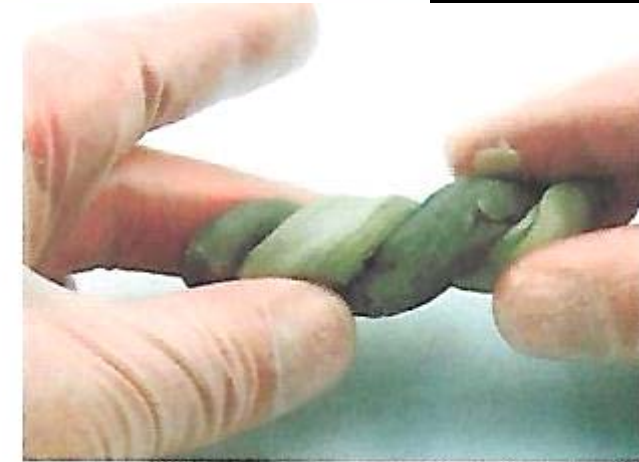
Part A and Part B are kneaded together by braiding and folding until colour is consistent.
