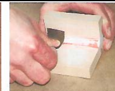
In making this inside corner, first body filler was used to build up the radius (left) and then a final layer of spot filler was used on top (middle) and sanded smooth (right).
