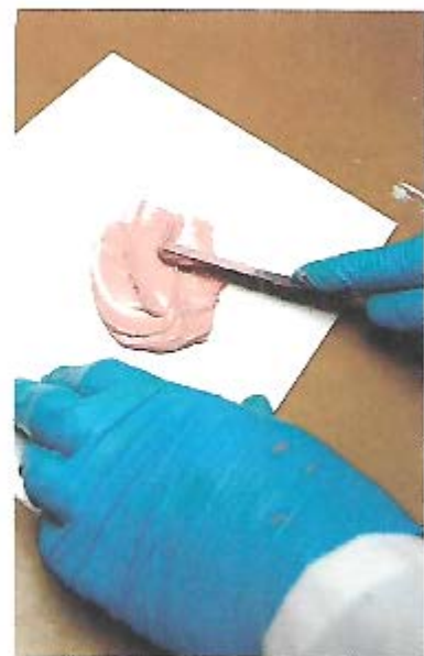
Automotive body filler is mixed according to the manufacturer's instructions. It is important to achieve a uniform colour consistency to ensure that mixing has been thorough.
