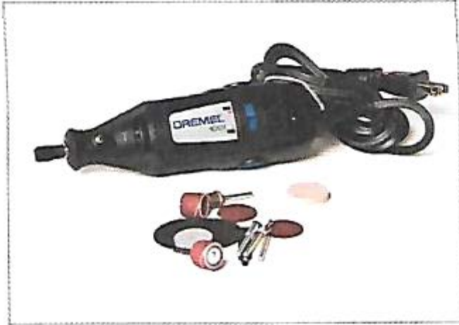
Rotary tools, such as this one made by Dremel, include a wide array of small bits suited to modelmaking work.
