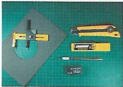
A Stanley knife and scalpel should be stocked with extra blades and used on a cutting mat.
