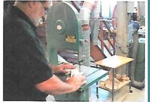
The bandsaw is a versatile shop tool for sawing straight as well as being useful for contoured cuts.
