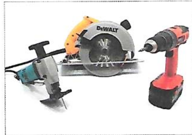
Hand-held drill, circular saw and jigsaw.
