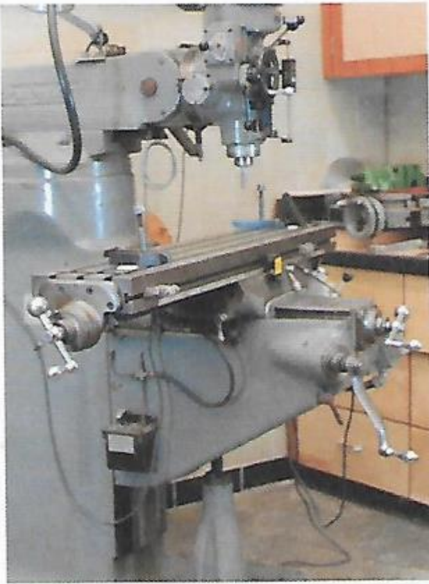
A knee mill can be used to create a variety of accurate cuts.
