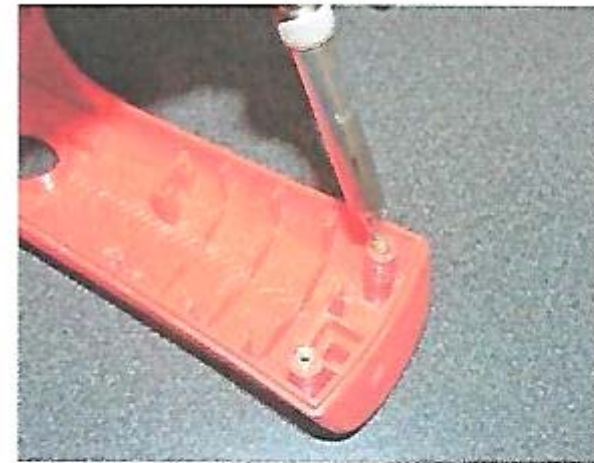
Rapid prototype parts can be fitted with threaded brass inserts. These allow easier opening and closing of the housing using machine screws.
