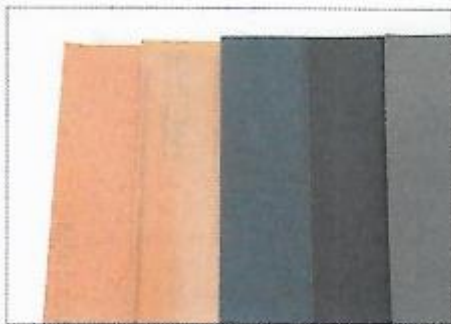
Different grit sandpapers are required for modelmaking. A basic toolset includes a range of coarse to fine sandpaper.
