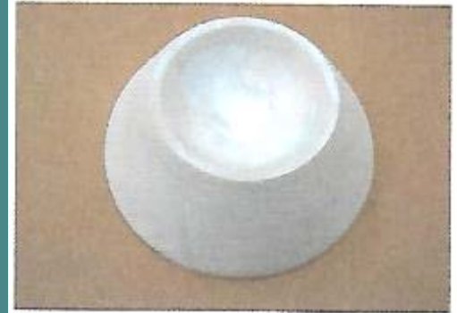
This bowl-shaped vacuum-forming mould was made on the wood-turning mill using a computer-generated template as a guide.
