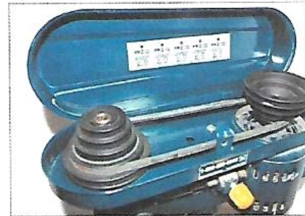
Drill press speed can be adjusted through a pulley arrangement between the motor and spindle. This should only be done when the machine is stopped and unplugged. The chart on the bottom of the guard cover on this machine shows speed options.
