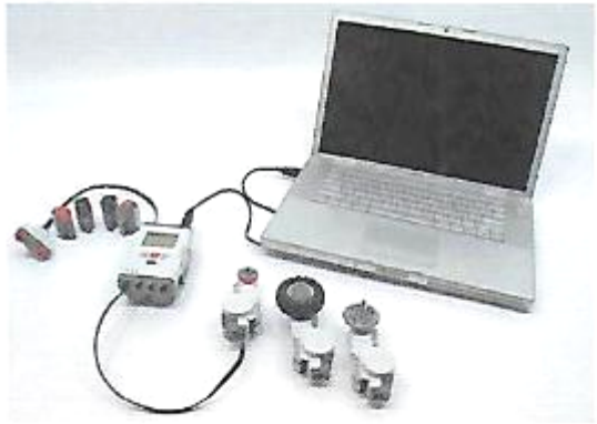
Lego Mindstorms® NXT is a stand-alone controller with an easily programmable interface. A variety of sensors, including touch, infrared, range and sound, can be used to produce output including servomotors. It is programmed through a computer.
