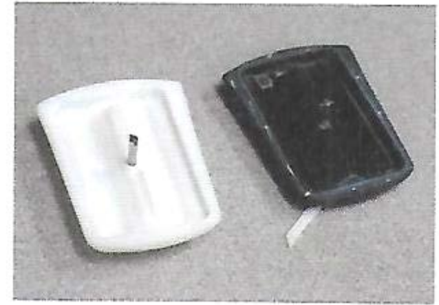
The new battery door (white) was printed on a Dimension 3D printer, based on data scanned in from the original battery door (black).
