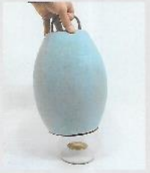
A Styrofoam look-alike prototype was used to determine the proper size and weight, despite the concern of if there it was too heavy and used. It was also possible to study the placement of the lantern on the ground and to be used.
