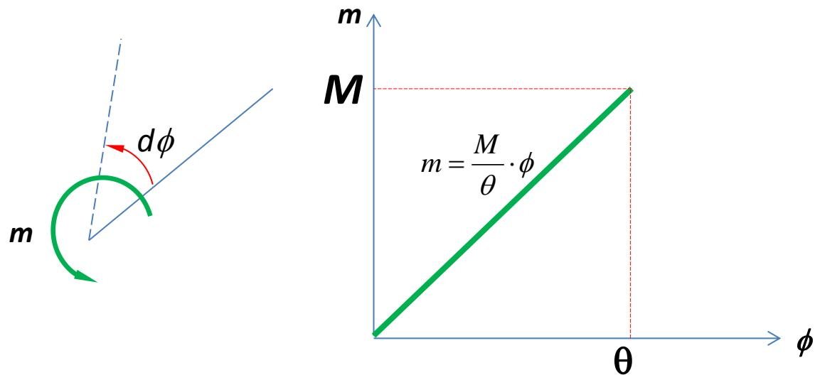
$$U_e = \int_0^\theta m \cdot d\phi = \int_0^\theta \frac{M}{\theta} \cdot \phi \cdot d\phi = \frac{1}{2} M\theta \quad (3)$$
