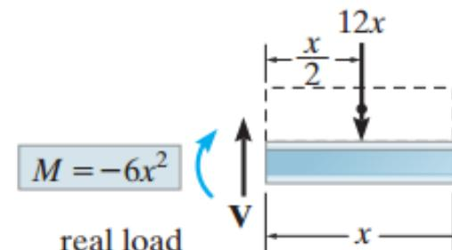
$$1 \text{ kN} \cdot \Delta_B = \int_0^L \frac{mM}{EI} dx = \int_0^{10} \frac{(-1x)(-6x^2)}{EI} dx = \frac{15.000 \text{ kN}^2 \cdot \text{m}^3}{EI}$$
