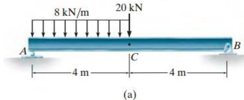
**External Force P.** A vertical force  $P$  is applied at point C. Later this force will be set equal to a fixed value of  $20 \text{ kN}$ .
