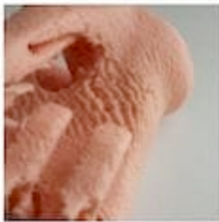
SIDE LAYER SURFACE ISSUES
